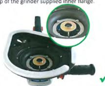
Never use the grinder supplied large cutting flanges! It will tear the rubber diaphragm.
