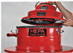
3. Place spacer sleeve and then position motor head and lock down with clamps.
